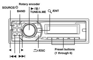
This unit cannot receive HD Radio signals (digital terrestrial radio). In order to activate the digital radio functions described below, an optional HD Radio Tuner module must be connected through the Ai-NET bus.
